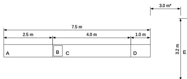
**Fig. 1** Walkway consisting of entry area (a); contact mat (b); data collection area (c); exit area (d); and projection screen (e). Asterisk distance between walkway and projection screen not to scale
