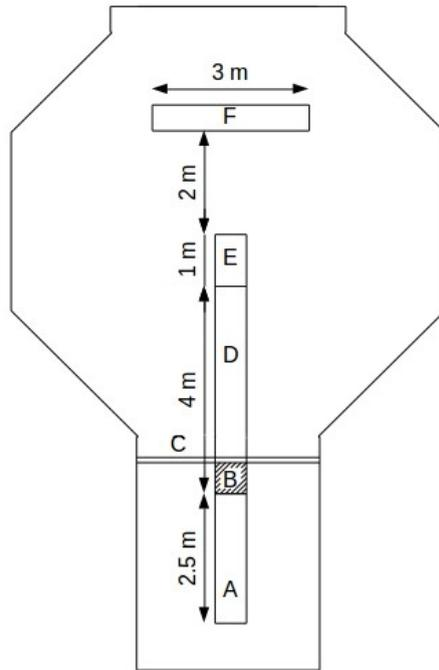
Figure 1: A schematic diagram of the experimental environment. The walkway into the waiting room consists of A: entry area, B: contact mat, C: sliding doors, D: data collection area, E: exit area, F: pedestrian area. All distances are to scale.
