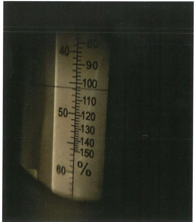
Fig. 2 100% of horizontal distance = 45 degrees
