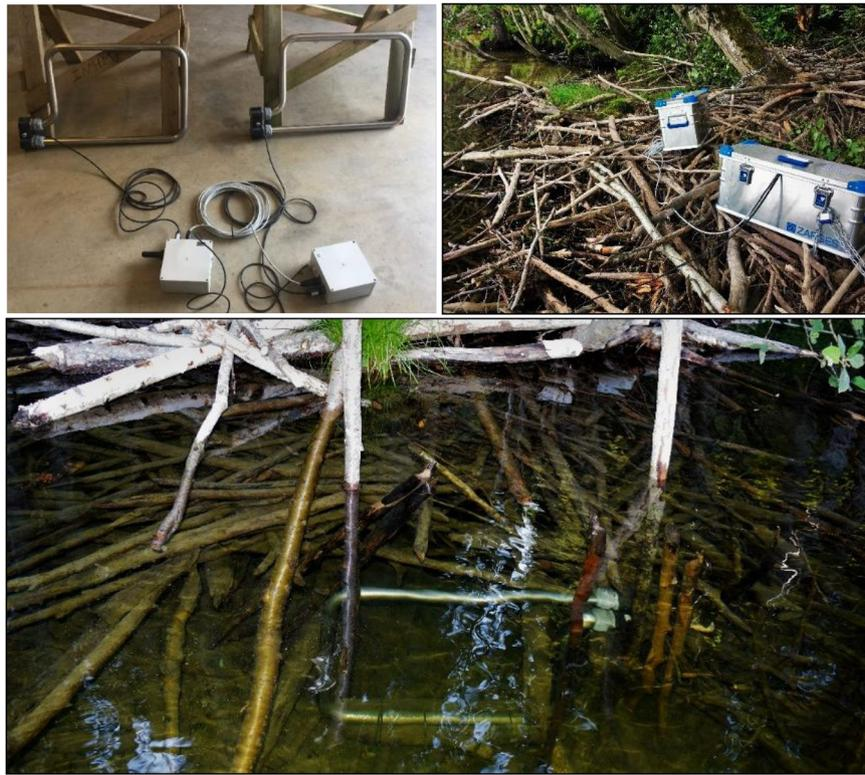
**Figure 3.** Photographs of the experimental radio-frequency identification set-up used to monitor Eurasian beaver in Norway during June 2018 to July 2019. (Top left) An automated, fixed-position passive integrated tag reader, with 2 loggers and corresponding antennas. The loggers were installed on the surface of the lodge in waterproof metal boxes (top right) and connected to underwater swim-through antennas attached to the lodge structure around entrance tunnels (bottom).
